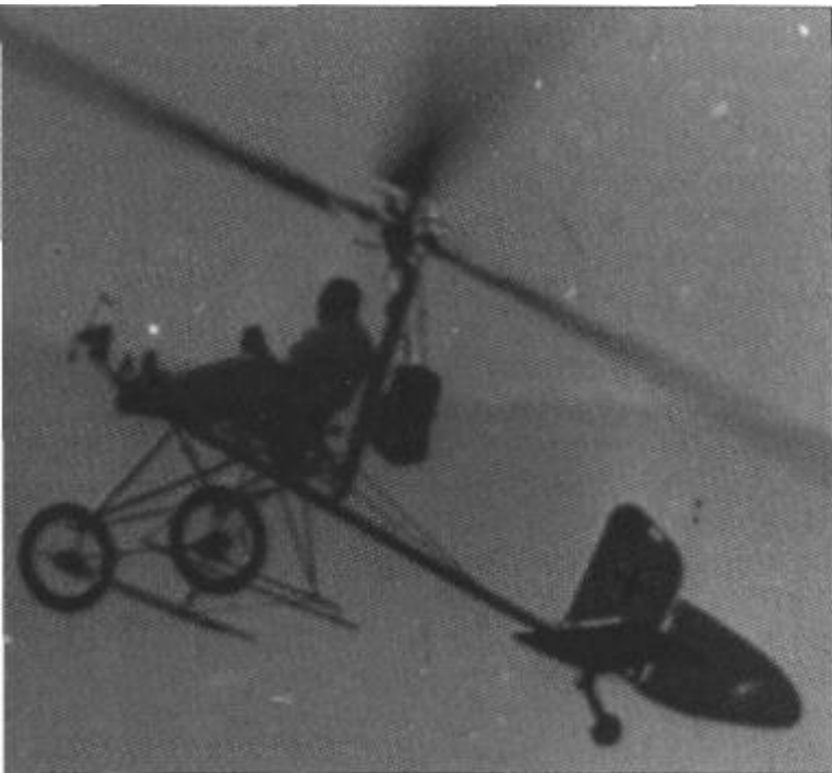
Above: The Fa 330 was not a true helicopter but an unpowered girokite; it was designed to be towed behind a submarine as an observation platform.
